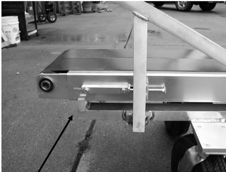
Note position of cart in relation to end roller assembly, never let conveyor roller assemblies rest on support bracket
